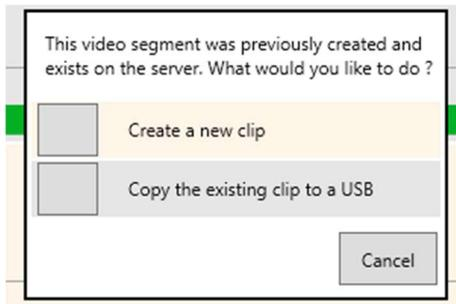
If the clip was previously created, you will be prompted to either create a new one or copy the existing clip to a USB drive. If you have a USB stick to copy the clip to, insert it and select this option.
